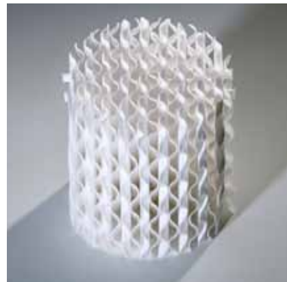
Structured packing made of PVDF in sheet structure, spec. surface area 300 m 2 /m 3 (packings with other specific surface areas available on request)
